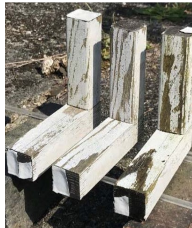
The acetylated L-joints after 20 years of exposure
